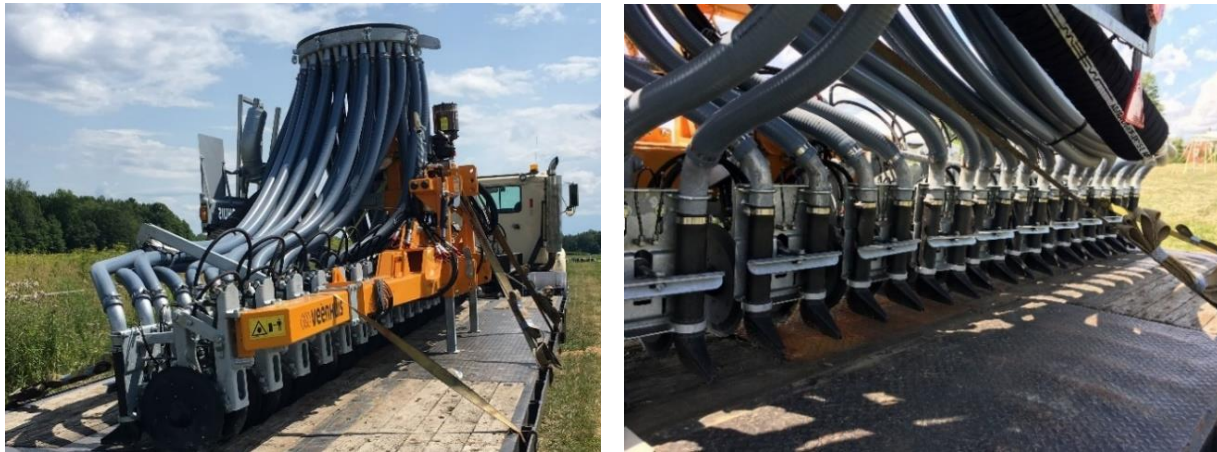
Figure 6. Grassland shallow slot manure injector to be used within the Lake Carmi watershed. Manure is injected subsurface to reduce surface runoff of nutrients. Equipment funds were awarded in SFY 2020 and will be reported in future Lake Carmi Clean Water Progress Report updates.
